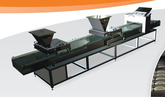
The Danielle Series of Linear Filling Machines is designed to automatically fill cardboard trays and paper baking cups with batter. The batter may be plain or include fillings such as fruit, nuts or chocolate chips. The machines are perfectly suitable for producing:
